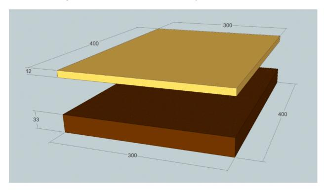
Usually I add 2 mm to the panel thickness. So I make maple panels 14 mm thick in order to get 12 mm after planing.
