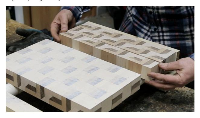
NB! Do not move the strips when clamping! Just slightly fix first two clamps. Then rotate the board, clamp another side and tighten all four clamps with the same pressure.
