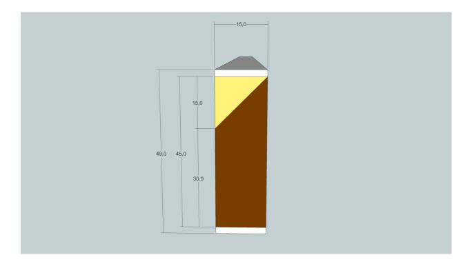
To make this part you should glue maple and walnut panels, cut the parts at table saw at 45 degrees and remove the reserves. We need 16 part, so it is necessary to make two 300 mm wide panels. The length of the panels should be about 400 mm. To be precise, the width of the panels may be only 235 mm, the length - about 200 mm. I made two 800 mm panels and finally got four cutting boards.
