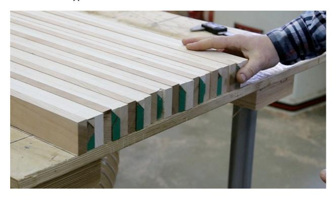
Glue three parts of each block. NB! Do not glue blocks to each other! In the video I clamp all eight blocks at once, but not glue blocks together.
