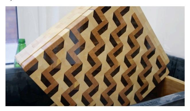
Then apply the hot mixture of mineral oil and beeswax (4:1 ratio)
