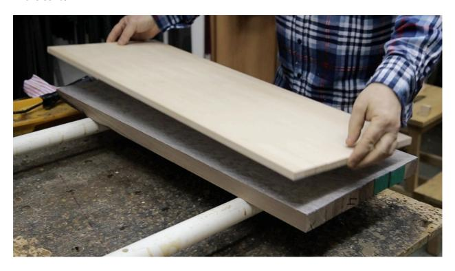
It is important to glue the panels well in the center. So use large F-clamps for this purpose. First clamp the panels in the center to squeeze out the excess glue, then clamp at the edges.
