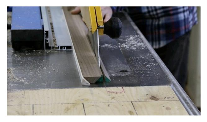
Divide 16 strips at two equal parts and make two types of blocks.
