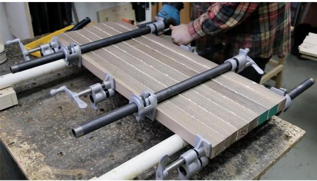
Wait a night and then plane the panels. You should be precise making this board. Make maple panels 12 mm thick.
