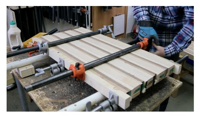
Next day plane the boards. Remove the reserves and make 45 mm thickness of boards. While planning the upper side of each board control the walnut corner.
