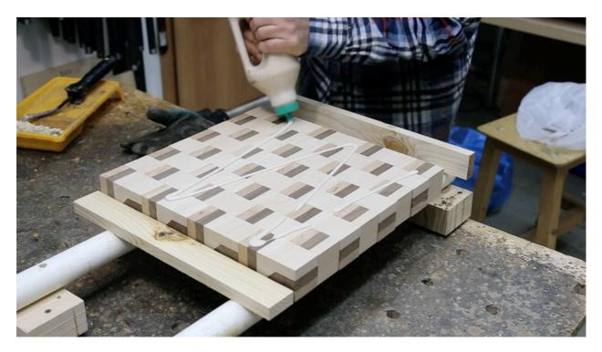
Glue also sacrificial rails. These rails will protect the cutting board edges while planning. Front rail is necessary to ensure a smoother entry the board into the planer. Back rail is needed in order to prevent tearing out the fibers at the exit the board from the planer.
