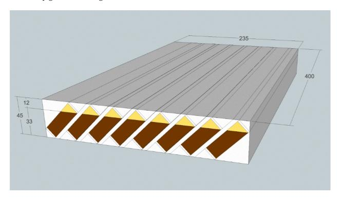
First you should make two maple panels 12 mm thick and two walnut panels 33 mm thick. The width of the panels must be about 300 mm, the length - 400 mm.
