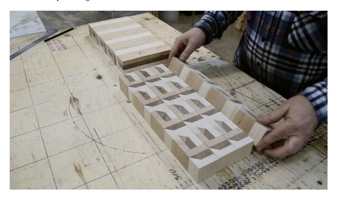
Assemble the cutting board.
